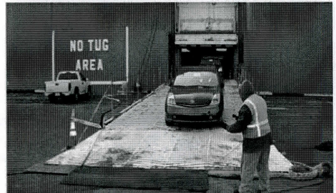
MONITOR DISCHARGE RAMP TO ENSURE NO BOTTOMING
