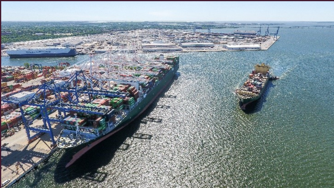
Photo: The Port of Baltimore’s fifty-foot shipping channel allows some of the largest, deep-draft ocean-going vessels to safely navigate into and out of the port. Photo Credit: John Wilhelm/Ports America Chesapeake
