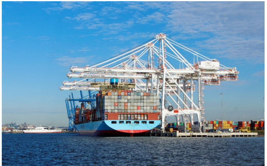
In October, the Helen Delich Bentley Port of Baltimore welcomed the largest container ship to ever visit Maryland. The Gunde Maersk, which has a capacity to handle 11,000 Twenty-foot Equivalent (TEU) containers was able to call the Port of Baltimore because of the Port's 50-foot deep channel and its supersized Neo-Panamax cranes.
