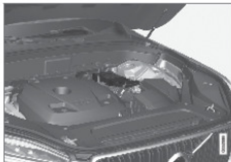
The support battery is located in the engine compartment, under the circuit breakers
