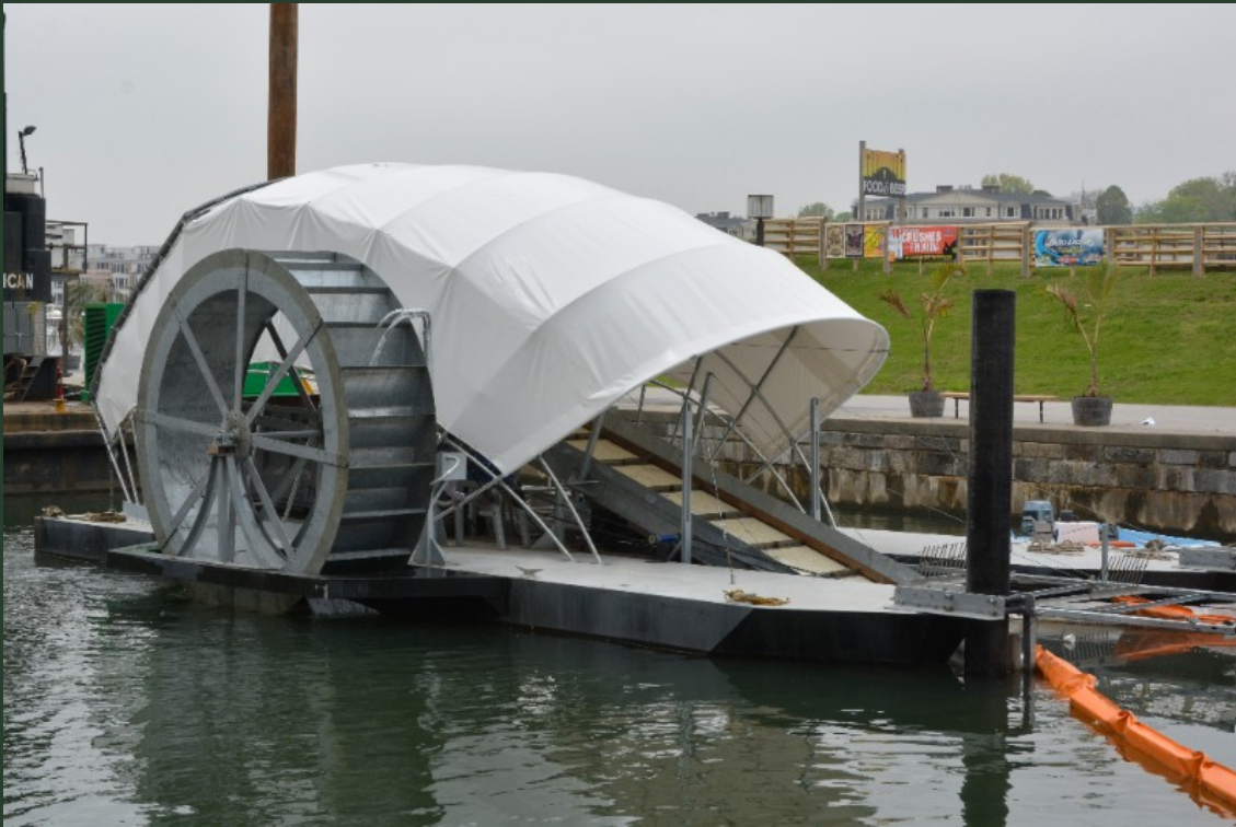
The MPA supports the operation of the Inner Harbor Water Wheel, which removes trash from the Jones Falls before it enters the Baltimore Harbor.
