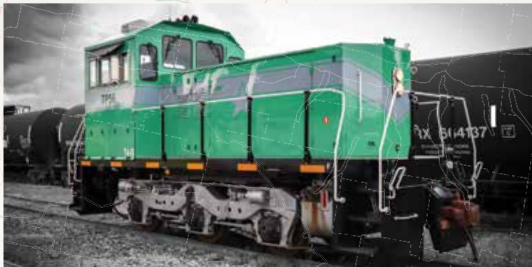
The TP56 from Tractive Power, equipped with a Tier 4 Final Engine
