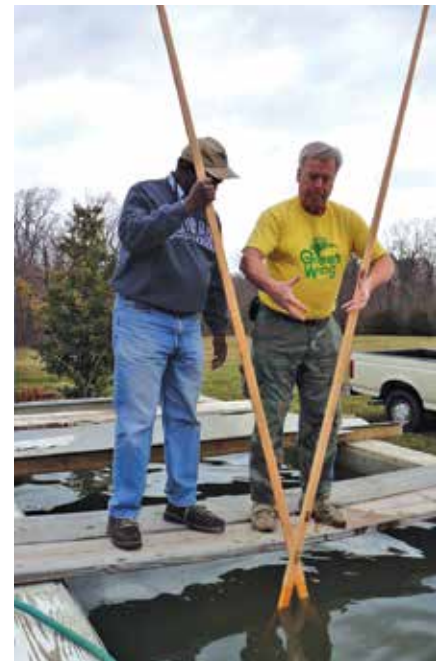
↑ The state is determining whether recycled concrete aggregate from highway projects can be used to create oyster reefs. Oyster growth and survival rates were compared in tanks. (Bottom right) Dr. Kelton Clark (left) works with a local waterman for oyster restoration.
