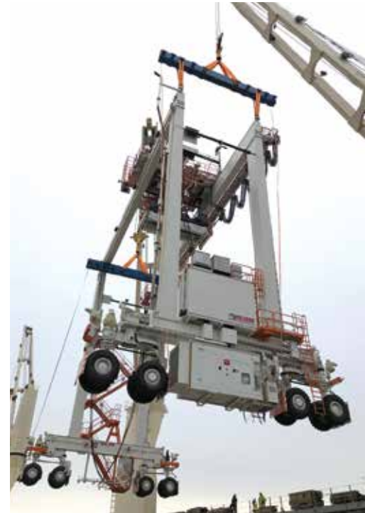
↑ One of the six Kalmar rubber-tired gantry cranes is lowered into place at Seagirt Marine Terminal this winter. Ports America Chesapeake now has 22 cranes at work.
